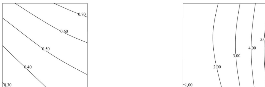
Fig. 1. Stresses in the plaster coating at temperature deformations under the influence of minus and plus temperatures, t/m^2
